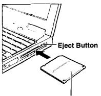
Label on the top surface, and insert the shutter-side headfirst.
